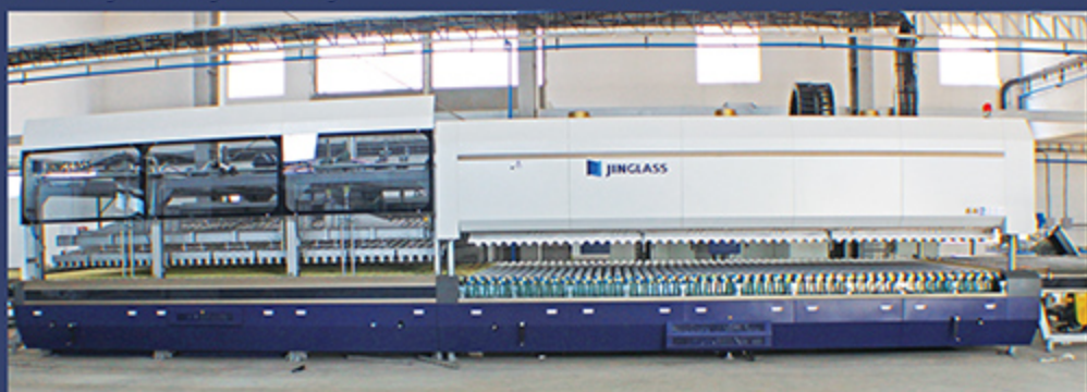
Forced Convection Tempering Line
